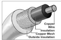
sists of an inner copper conductor surrounded by a braded or mesh shield. The shield, in turn, must be electrically connected to the earth. This enables the
